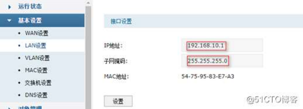
图20. 网关TL-ER3210G的LAN口配置
