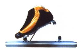
Unlike conventional skates, the heel of the clap-skate blade is not attached to the boot, and the toe of the blade is affixed to the boot with a hinged apparatus. At the end of each stride, as the skater picks up the skate, the blade briefly disconnects from the heel of the boot, thereby keeping the blade on the ice longer and increasing the skater's pushing power. When the blade has fully extended, a spring mechanism mounted on the
