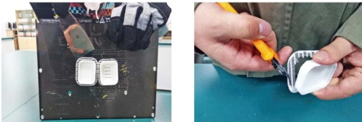
图7-4-32 剥离底座及去除支撑
