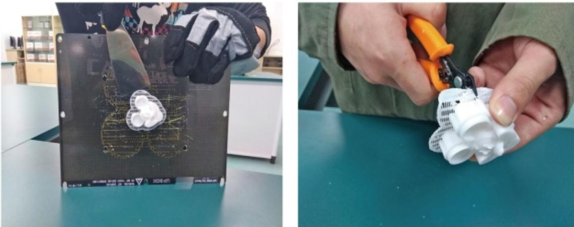
图7-5-39 剥离底座及去除支撑
